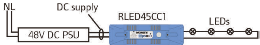
Single channel constant current 45W LED dimmer
